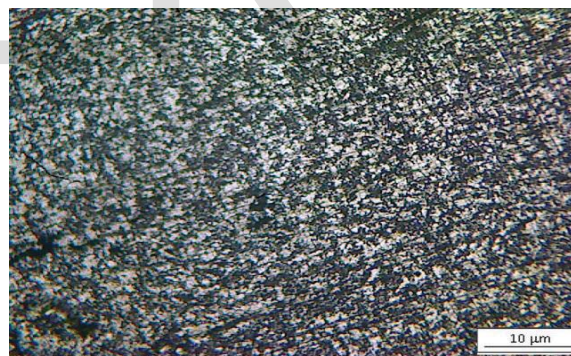
Fig .10 - microstructure of Conventional Quenching
